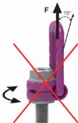
Pic. 6: Forbidden turning direction at loading in the direction of the axle.
