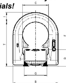
7. The lifting point is suitable for use within temperature range -20°C up to 400°C. For use within the following temperature ranges the WLL must be reduced by the following factors:
